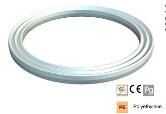
Connection thread sealing ring, in accordance with Part 9 to DIN 46320, however, dimensions may, according to material or function, deviate, suitable for all plastic cable glands with PG connection thread to DIN EN 40430, the internal diameter of the sealing rings are designed so that they can be captively premounted.
