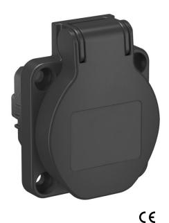
Protective contact extension socket 0° with hinged cover, with screwless terminals, 2-pin, 16 A, 250 V~, with connection terminals to IEC 60884-1. Protection rating: IP44.
