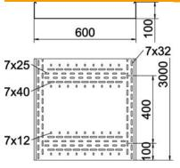
Length 3,000 mm Length 10 ft Width 600 mm Width 24 in Height 100 mm Height 4 in Plate thickness 0.08 in Plate thickness 2 mm Dimension B 600 mm Dimension H 100 mm Dimension L 3,000 mm
