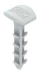
Push-fit plug Delta-Push® for mounting electrical installations. Suitable for concrete, calcareous limestone, full brick, hollow brick and porous concrete. Toolless mounting by pushing into a drill hole in a wall or on a ceiling. Without screws. To install cable trunking or labelling panels, for example.
