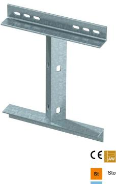
Adapter plate with slots for universal fastening to vertical steel girders and walls. Wall and support brackets are screwed to the adapter plate at a  $45^{\circ}$  angle. To support cable support systems in building corners and jumps. The hexagonal bolts, type SKS 12 x 40 GF, are used to fasten the brackets to the adapter plate. Please order the appropriate quantity.
