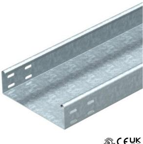
MKSU 60 = medium-duty cable tray system, unperforated, with a side height of 60 mm. Straight connectors should be ordered in the appropriate quantity. The cable tray has connector perforations on both sides. Magnetic shield insulation without cover 20 dB, with cover 50 dB.
