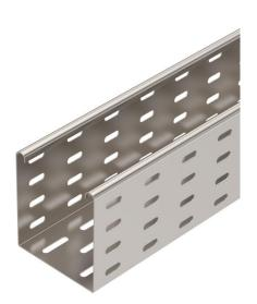
MKS 110 = medium-duty cable tray system with a side height of 110 mm. The cable tray is fastened to the bracket with screws, type FRS M6 x 12. Magnetic shield insulation without cover 20 dB, with cover 50 dB.
