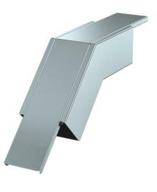
45° vertical bend, falling version, with intumescent fire protection mesh for PY-ROLINE® Rapid PLM installation duct. Suitable for direct wall and ceiling mounting, mounting below system floors and on support systems. Tool-free joint mounting with PLM SI joint connector. The cover is snapped on without tools, allowing rapid inspection and retroassignment. The cover overhang allows offset cover mounting for continuous equipotential bonding of the entire duct section.
