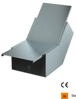
45° vertical bend, rising version, with intumescent fire protection mesh for PYRO-LINE® Rapid PLM installation duct. Suitable for direct wall and ceiling mounting, mounting below system floors and on support systems. Tool-free joint mounting with PLM SI joint connector. The cover is snapped on without tools, allowing rapid inspection and retroassignment. The cover overhang allows offset cover mounting for continuous equipotential bonding of the entire duct section.
