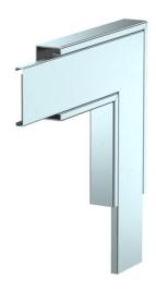
Flat angle with intumescent fire protection mesh for PYROLINE® Rapid PLM installation duct. Suitable for direct wall and ceiling mounting, mounting below system floors and on support systems. Tool-free joint mounting with PLM SI joint connector. The cover is snapped on without tools, allowing rapid inspection and retroassignment. The cover overhang allows offset cover mounting for continuous equipotential bonding of the entire duct section.
