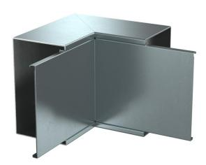
Internal corner with intumescent fire protection mesh for PYROLINE® Rapid PLM installation duct. Suitable for direct wall and ceiling mounting, mounting below system floors and on support systems. Tool-free joint mounting with PLM SI joint connector. The cover is snapped on without tools, allowing rapid inspection and retroassignment. The cover overhang allows offset cover mounting for continuous equipotential bonding of the entire duct section.
