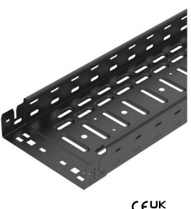
Cable tray with integrated quick-fastening system. Strip-galvanised surface, visible areas powder-coated in jet black (RAL 9005). Continuous side perforations of 7 x 20 mm for the installation of additional connection and mounting components. With 11 mm perforation in the base for direct threaded rod suspension. Usable length 3,000 mm.
