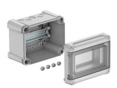
Distribution box with terminal strip for surface mounting, for the current sub-distribution in interior and exterior areas, in accordance with IEC 439-3. With premounted 35 mm hat profile rail. IP66 protection type and IK08 protection rating. Transparent cover to screw on, with cut-out. Including 4 screw cover caps.
