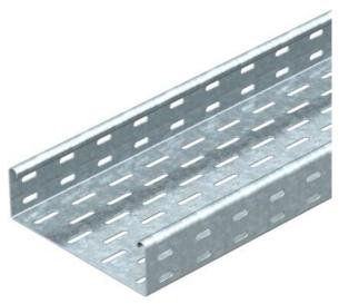
SKS 60 = heavy-duty cable tray system with 60 mm side height. The cable tray, type SKS, should also be used for the maintenance of electrical function. For additional data, please refer to BSS fire protection systems. Magnetic shield insulation without cover 20 dB, with cover 50 dB.
