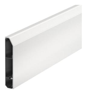
SL skirting trunking for covered cable routing in internal areas. The colour of the trunking bases can vary depending on the production method. With snap-on cover and base, with base perforation for direct wall mounting. Change the direction with the fittings and close the trunking ends with end pieces. Service outlet for installing power and data technology. Tested according to DIN EN 50085-1 and DIN EN 50085-2-1. Base and cover packed as a set in a box. The trunking couplings must be orde-
