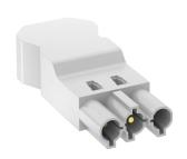
Connector part, 3-pin, type GST18i with screw connection for cables of 1.5–4.0  $\,$  mm² and cable diameters between 10.5–14.5 mm (H05VV, NYM), unmounted with strain relief, terminable in situ, 250 V, 16 A.
