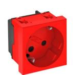
Protective contact socket Single 33°, encoded version, with increased touch protection, with screwless terminals, 2-pin, 16 A, 250 V $\sim$ , with connection terminals according to IEC 60884-1.
