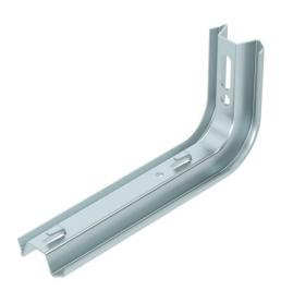
TP bracket with clamping lugs for screwless mesh cable tray fastening. If the bracket is fastened directly to the wall or the profiles are screwed together, then, for reasons of stability, always use the spacer, type DS 4. Mesh cable trays with a 50 x 100 mm grid width, e.g. type GRL, GR and GRM, can be fastened to the TP bracket without screws.
