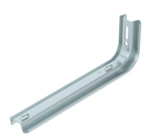
TP bracket with clamping lugs for screwless mesh cable tray fastening. If the bracket is fastened directly to the wall or the profiles are screwed together, then, for reasons of stability, always use the spacer, type DS 4. Mesh cable trays with a 50 x 100 mm grid width, e.g. type GRL, GR and GRM, can be fastened to the TP bracket without screws.
