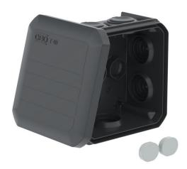
Junction box for the connection of cables indoors and in protected outdoor areas. Square design with plug-in seals to the sides and knock-out entries in the bottom. Suitable for wall and ceiling mounting and on mounting panels. With the option to fasten inside. With fixed clamping cover. Made from halogen-free, UV-resistant materials.
