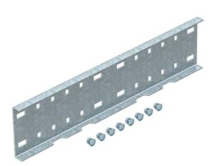
Longitudinal connector for the connection of wide span cable trays and ladders of type WKSG and WKLG with a side height of 110 mm. Including appropriate bolts and combination nuts.
