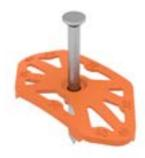
Nail-Fix nail clip with pre-mounted galvanised steel nail, to fix cables in wall slots of between 25 mm and 46 mm width and on masonry.
