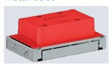
Underfloor outlet box with fixed, unchangeable  $106 \times 182$  mm installation opening for an installation unit of nominal size 2. The mounting opening is created using the screed protection cover contained in the scope of supply. The underfloor box has two openings for M20 conduit on the narrow sides. The underfloor box is suitable for screed floor constructions with height 70 mm up to 90 mm.
